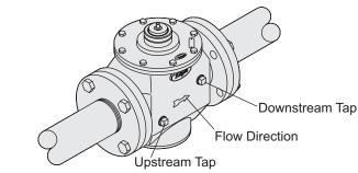
VALVE/PIPE CONNECTIONS (2-1/2" THROUGH 3" SIZES, Weld-ON FLANGES)
